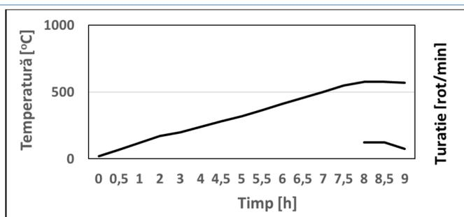
Figure 1. Pre-melting-melting-refining-homogenization program according to the invention, comprising temperatures, time frame, mixing regime, for BPPG3Ce composite.
