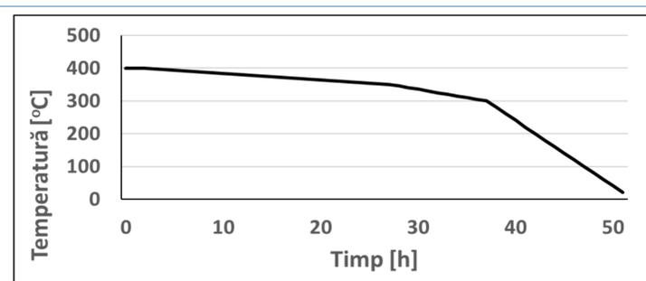
Figure 2. Annealing program for BPPG3Ce composite according to the process proposed in the invention, comprising the temperatures and time frame of the annealing process steps.
