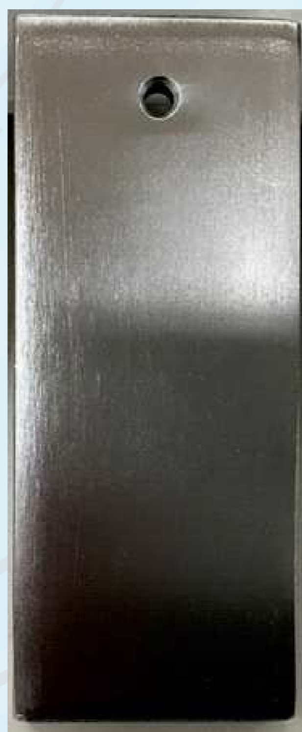
(b) Electrodeposition of the zinc-nickel alloy by the claimed method, on stainless steel substrate
