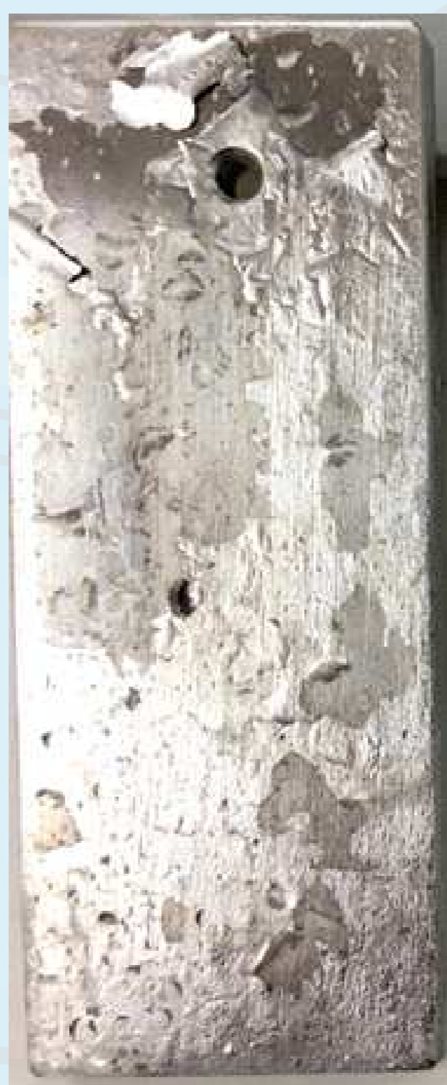
(a) Electrodeposition of the zinc-nickel alloy without using the method claimed on stainless steel substrate.
