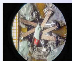
Fig. 8 Test setup for measuring the temperature gradient \Delta T of thermoelectric materials.
