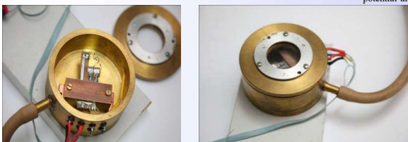
Fig. 7. Test device for measuring the temperature gradient \Delta T of low dimensional thermoelectric materials
