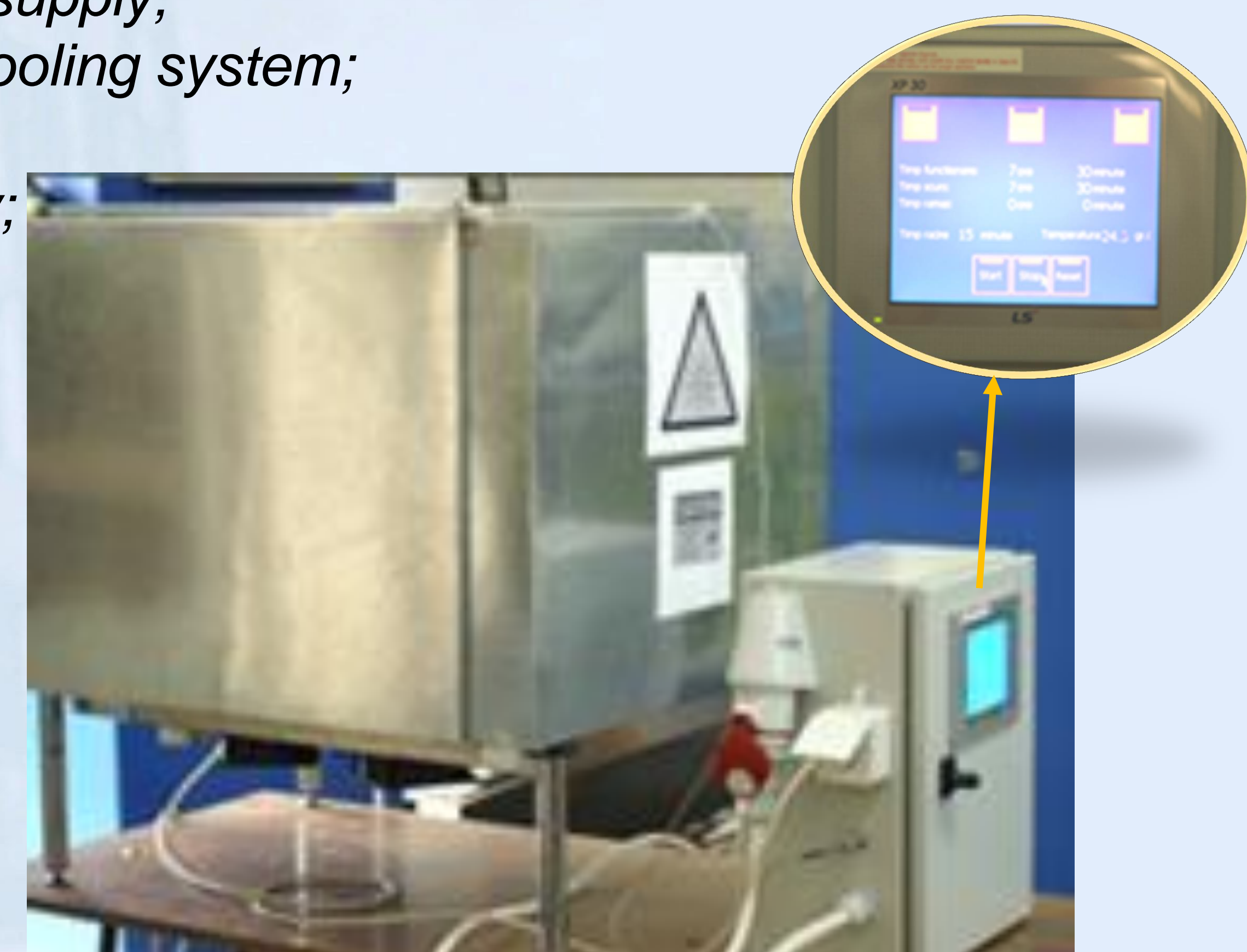
Figure 2 - Monitoring and control system for UV artificial ageing of thermoplastics and composites
