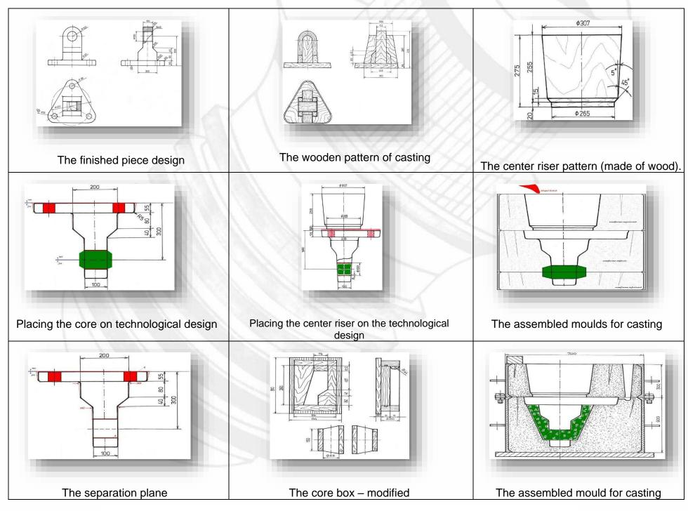
Application in industrial practice of all the technological method applied lead to the decrease the percentage of rejects registered from 13% to about 4%. This aspect has a positive influence in castings costs respectively in the company costs.
