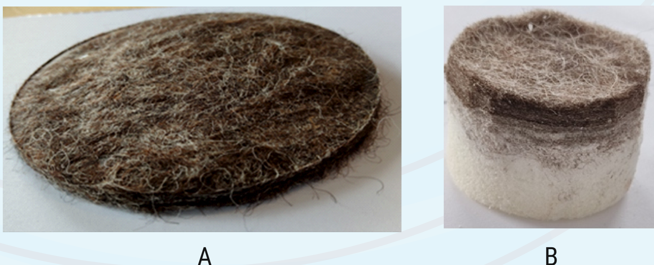
Fig.1. Processing phases: A: Phase I - Wool plate hot formed ; B: Phase II - Finale structure of the plate
