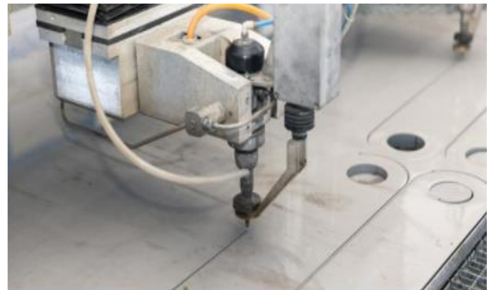
Waterjet cutting operations with complementary Garnet abrasive
