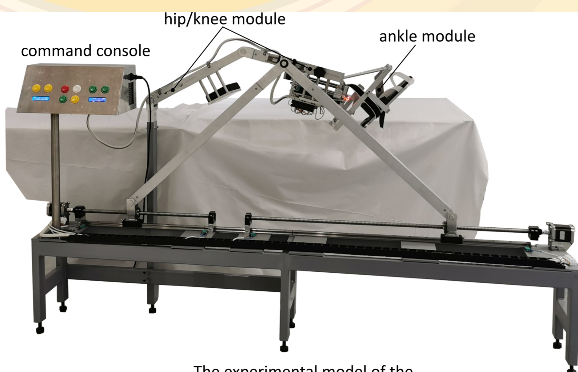
The experimental model of the RECOVER parallel robot for lower limb rehabilitation
