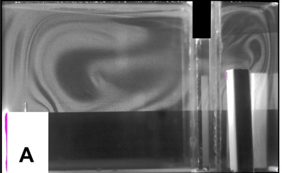
The second recording system – arranged vertically – uses Schlieren techniques and consists of a point light source, two parabolic mirrors, a shutter, a high-speed video camera and a computer. The role of this system is to highlight the initiation of the explosive atmosphere inside the transparent construction and the development and behavior of the flame front during the explosion process.
