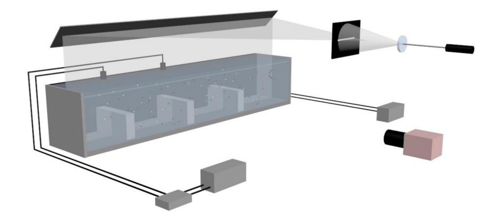
The problem solved by the invention consists in the possibility of analyzing the explosion phenomena of air-fuel-fuel mixtures at higher recording speeds of parameters and at relatively low costs due to the simplicity of the system components, its ability to record gas explosion phenomena from the moment of the initiation of the explosive atmosphere until the development of the flame front and the passage of the flow in turbulent regime.
