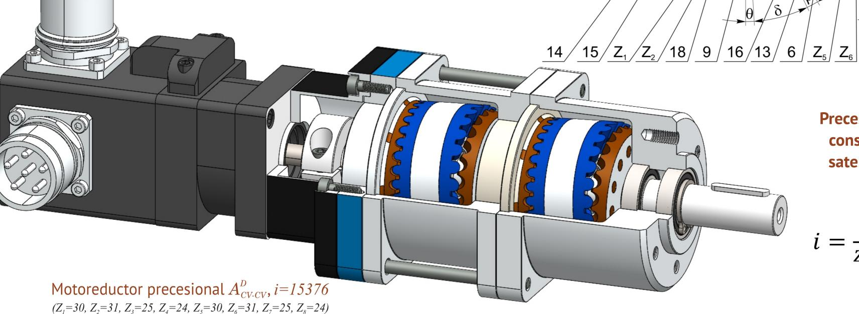
Precessional transmissions with two consecutively coupled semi-crank satellites  $(\pm 3600 \le i \le \pm 12.96 \cdot 10^6)$
