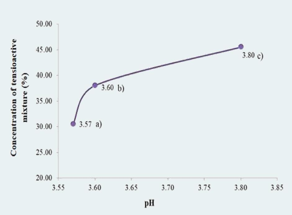
pH values for the invented microemulsions, coded MEAS1, MEAS 2 and MEAS 3, as a function of the selected tensioactive mixture
