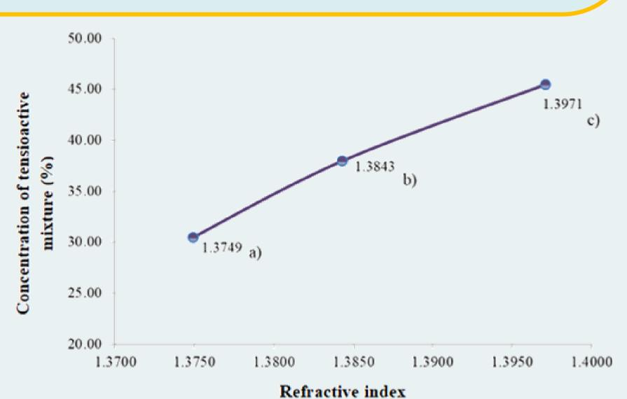
Values of refractive index expressed as a function of the tensioactive mixture content for the invented microemulsions, proving the isotropic character
