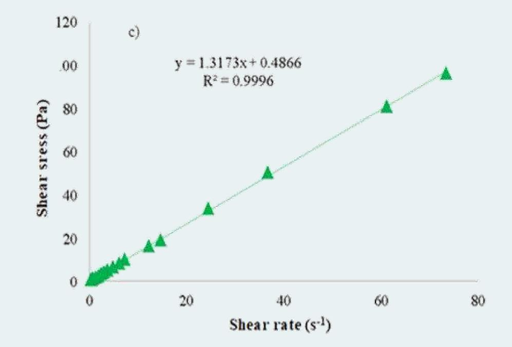
Rheological profiles for the invented microemulsions MEAS 1 (a), MEAS 2 (b) and MEAS 3 (c), expressed as shear stress versus shear rate, defining the linear character according to Newton's law
