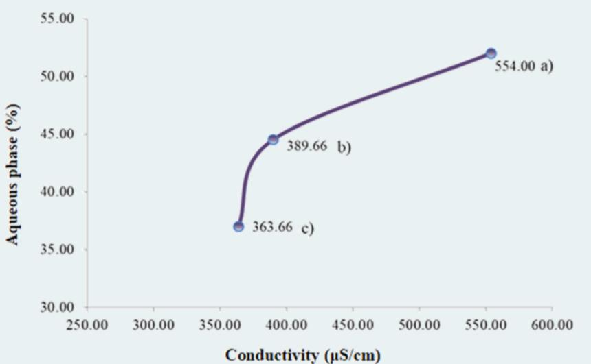
Conductivity values ( $\mu$ S/cm) for the invented microemulsions as a function of the aqueous phase content, defining the oil in water type of microemulsions
