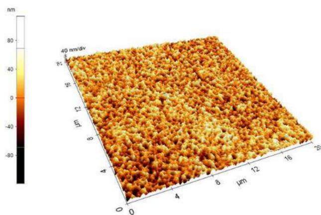
**Figure 1.** AFM image of the 1.5% rGO/ $\text{TiO}_2$ / $\text{P}_2\text{O}_5$  film
