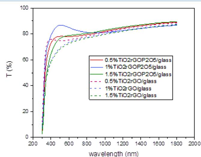
**Figure 3.** UV-Vis-NIR spectra of  $\text{TiO}_2$ /rGO and  $\text{TiO}_2$ rGOP $_2$ O $_5$  thin films on glass substrate at different concentrations of rGO in precursors mixture solutions.
