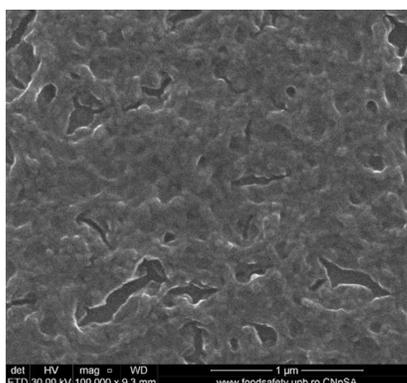
**Figure 2.** SEM image of the 1.5% rGO/ $\text{TiO}_2$ / $\text{P}_2\text{O}_5$  film
