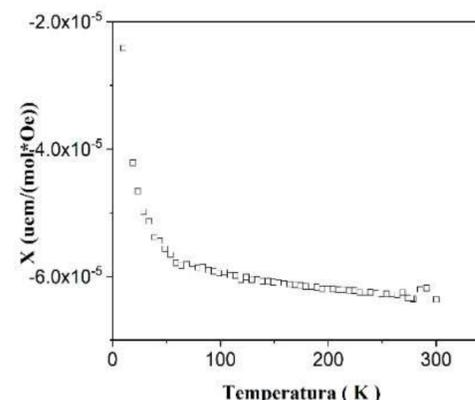
Figure 2. Magnetic susceptibility depending on temperature
