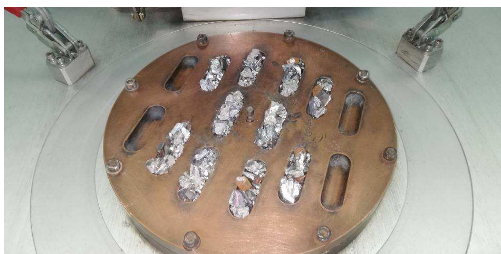
Water-cooled copper plate in which the metallic materials of the load are placed in order to melt high entropy alloys under an inert argon medium in the RAV installation.
