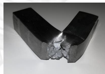
Aspect of high resilient weld
